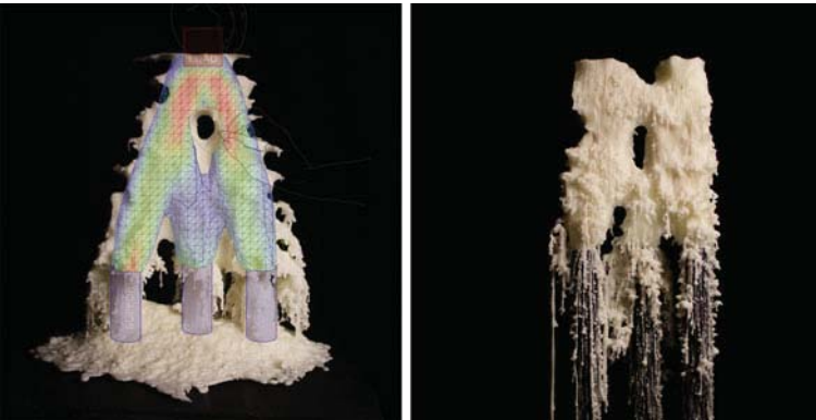
Fig. 7 Left topologically optimized digital model versus materially informed result. Right iteratively melted form with two loading points, three supports, and user indicated void
