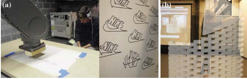
Fig. 3 Left a Human as noise generator: the robot’s level of precision while drawing is linked to the real-time values of an EEG headset, such that the drawing becomes messier as the human loses focus. Right b [AR]chitecture: gesturally defining a loft surface and a brick wall simultaneously using the Kinect (Johns 2012)
